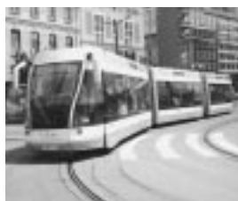
Fig.10 A rubber-tired tram that can operate without a guide rail (Nancy, France)
