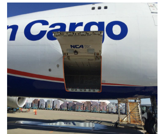
LOWER DECK FORWARD CARGO DOOR
